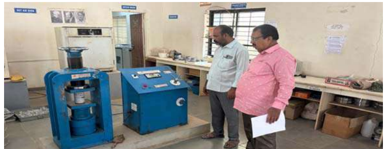
CC Cores testing at CETL-ESCI on GHMC-TPQC for Road works
